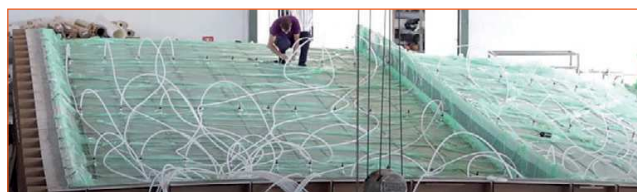
Fig. 2: Infusion process for one of the 240 sqm composite canopy's sections
